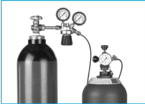
The use of pre-loading set for the inflation of accumulators "low pressure" series requires, for safety reasons, the use of a **pressure reducer mounted on the nitrogen bottle** calibrated at a pressure equal or lower than the max working pressure PS marked on the accumulator body. The connection nipple between charging hose and reducer it is showed by the side of the page and it is normally supplied with the pre-loading set.
