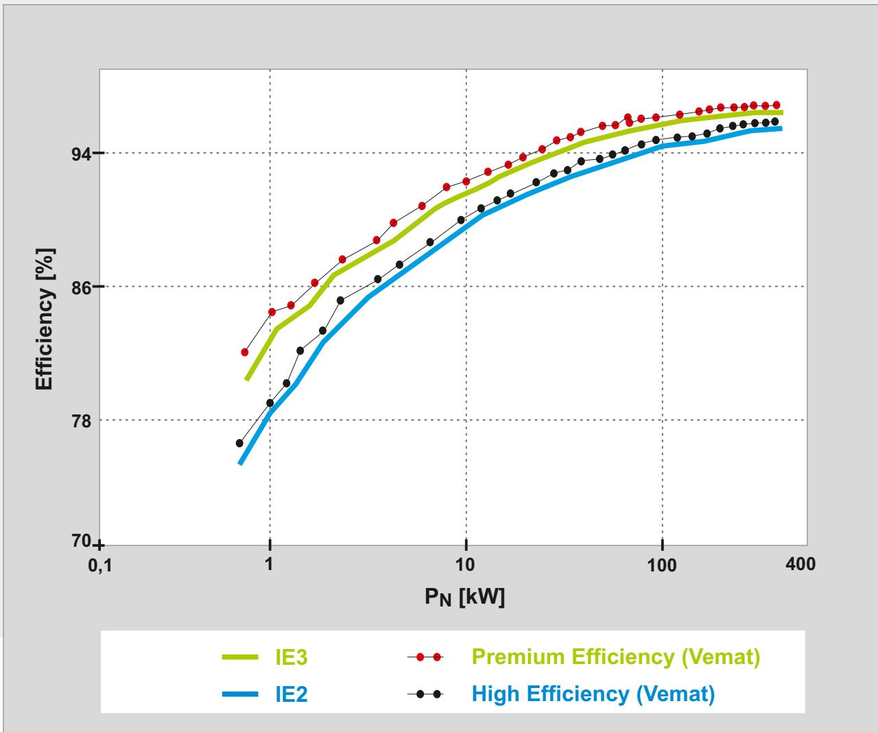
The efficiency class system specified under IEC 60034-30-1 is valid for low voltage three phase squirrel cage induction motors with the following specifications:
