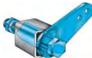
Fig. 14 Lever connection with one through bolt
