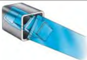
Fig. 13 Plug-in connection with lever and welded-on square steel piece
